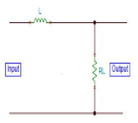
This type of filter is also called choke filter. It consists of an inductor L which is inserted between the rectifier and the load resistance R<sub>L</sub>. The rectifier contains A.C components as well as D.C components. When the output passes through the inductor, it offers a high resistance to the A.C component and no resistance to D.C components. Therefore, A.C components of the rectified output is blocked and only D.C components reached at the load.
