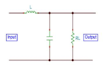
In inductor filter, the ripple factor is directly proportional to the load resistance. On the other hand in a capacitor filter, it is varying inversely with the load resistance. Hence if we combine the inductor filter with the capacitor the ripple factor will become almost independent of the load filter. It is also known as inductor input filter, choke input filter, L input or LC-section.
