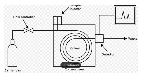
• Sample which is to be separated is mixed with appropriate volatile solent such as heptane, acetone or methanol, just before the column there is a septum (injector) which inject the sample to the column, Temperature of the injection tegion is kept 20 to 50 degree celcius higher than the column, this allows the rapid volatilization of the sample. once the sample volatilized, it persist on the column where the separation occurs.
