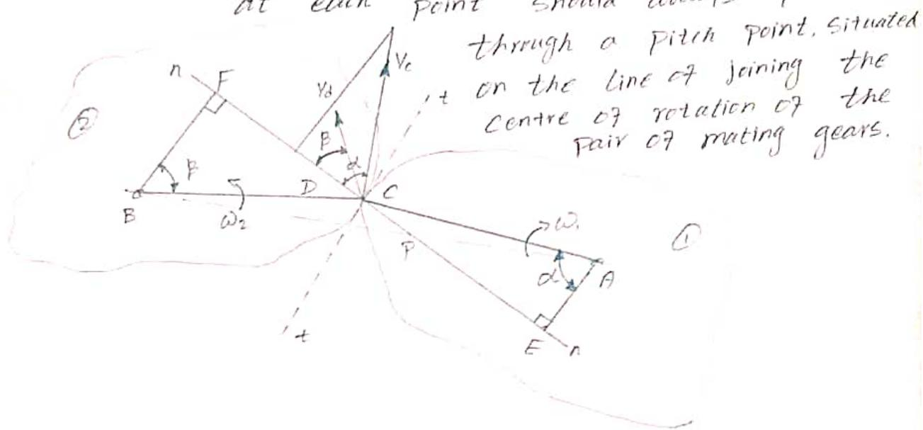
through a pitch point, situated on the line of joining the centre of rotation of the pair of mating gears.
