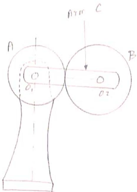
In the above figure, gear A and the arm C have a common axis at  $O_1$ , about which they can rotate. The gear B meshes with gear A and has its axis on the arm at  $O_2$  about which the gear B can rotate. If the arm is fixed, the gear train is simple and gear A can drive gear B or vice-versa.
