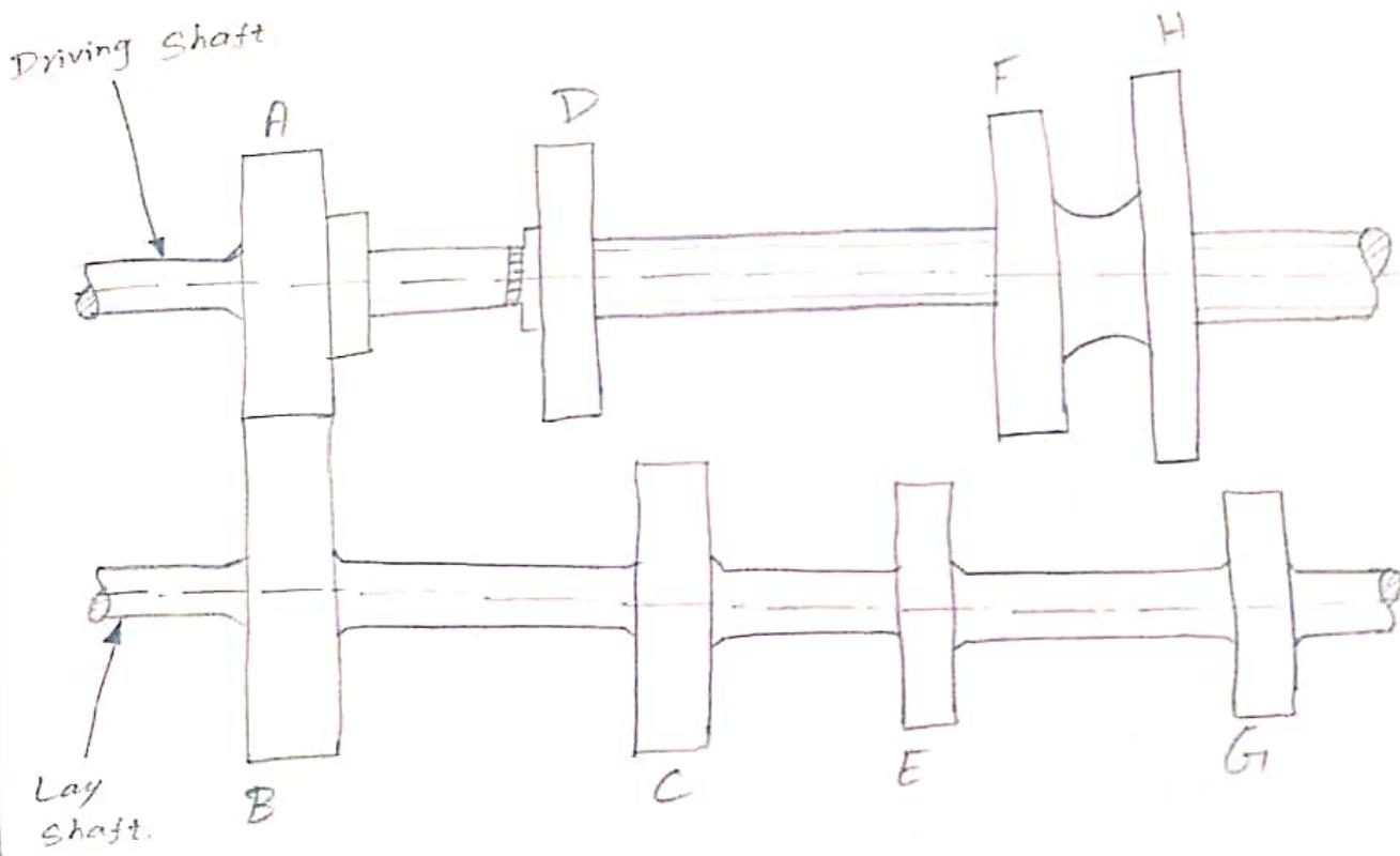
The above figure shows the gear box is in the neutral position. The pinion 'A' is keyed to the driving shaft is in constant mesh with the gear 'B' on the lay shaft. The gears B, C, E and G are rigidly fixed on the lay shaft.
