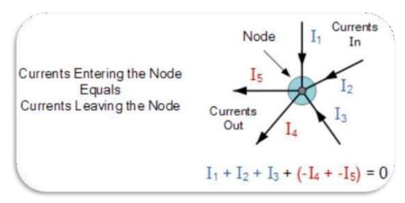
Here, the 3 currents entering the node, I<sub>1</sub>, I<sub>2</sub>, I<sub>3</sub> are all positive in value and the 2 currents leaving the node, I<sub>4</sub> and I<sub>5</sub> are negative in value. Then this means we can also rewrite the equation as;
