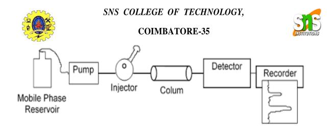
High pressure pump pumps Solvent (Mobile phase) in to the column and the Sample molecules are injected into the column ,the sample molecules are separated in the column and is detected by the detector and the peak is obtained on the computer ,this peak is plotted with respect to the retention time.
