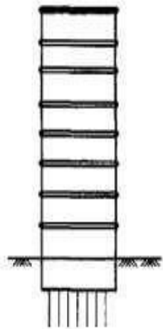
A multi-storied building on piles
