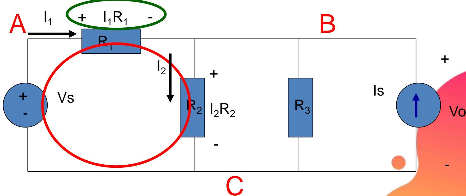
Starting at node A, add the 1<sup>st</sup> voltage drop:  $+ I_1 R_1$
