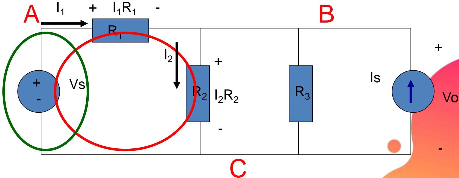
Subtract the voltage rise from C to A through  $V_s$ :  $+I_1R_1 + I_2R_2 - V_s = 0$
