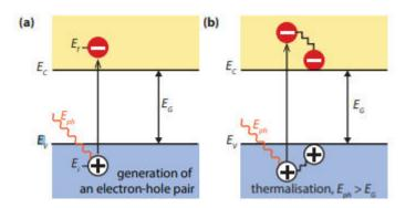
populated by electrons. Hence, this energy difference is called the bandgap, EG = EC - EV. If a photon with an energy smaller than EG reaches an ideal semiconductor, it will not be absorbed but will traverse the material without interaction.
