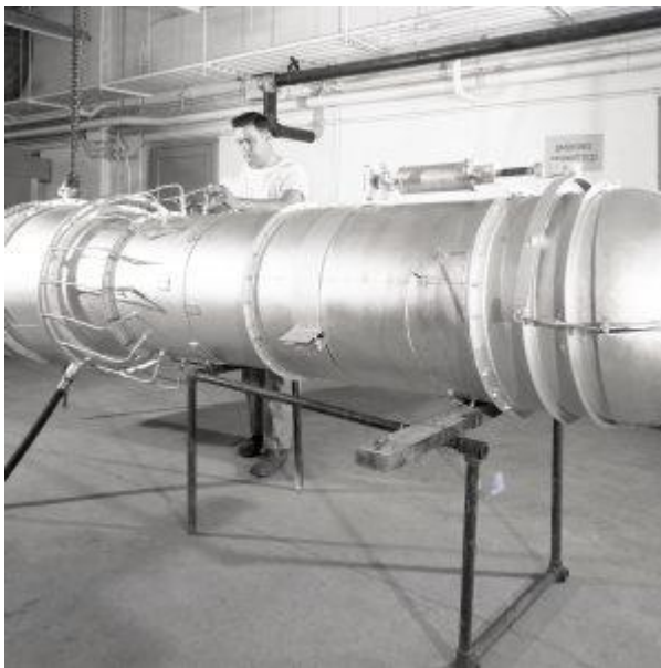
A tailpipe with variable-area nozzle for a General Electric TG-180 in the JPSL (1946).
