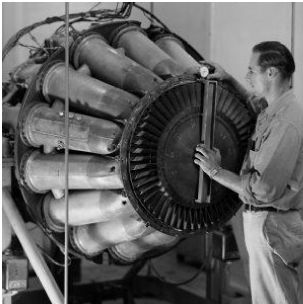
A mechanic checks out a GE I-40 engine equipped with a tailpipe burner (1946).
