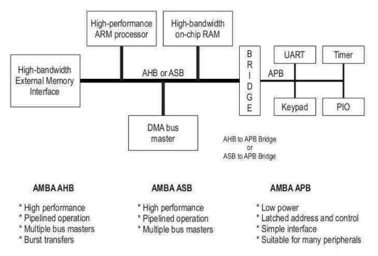
AMBA stands for Advanced Microcontroller Bus Architecture. AMBA specification specifies an on chip communication standard. This is used to design embedded microcontrollers with high performance.
