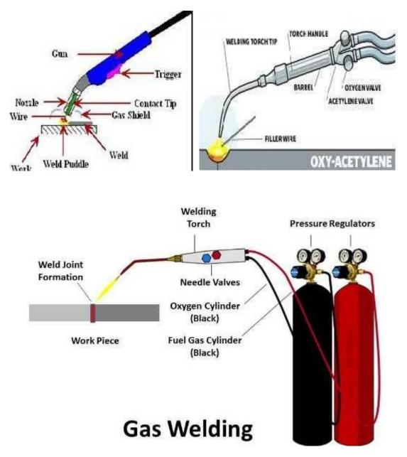
**GAS WELDING**: 1.Oxy – acetylene welding 2) Oxy – hydrogen welding 3) Air – hydrogen
