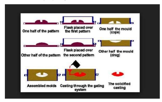
t. The mould is ready for pouring the metal.
