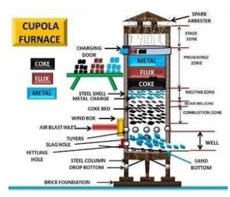
**<u>Preparation</u>**: The slag and waste from previous melting are cleaned. Broken bricks are repaired or replaced if necessary. The bottom doors are closed. A sand bed with sloping towards tap hole is prepared upto a height of 200mm. A tap hole is formed and lined with clay. Then a slag hole is prepared. Finally the cupola is dried thoroughly.
