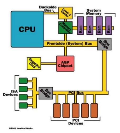
•The PCI Bus was originally 33Mhz and then changed to 66Mhz.
