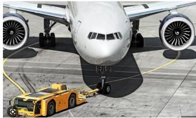
DEFINITION Towing is the process of moving the aircraft without using engine power by pushing by hands or using tow bar and tow tractor.
