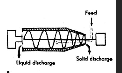
• Feeds with high solids contents are separated using desludging centrifuges, including conveyor bowl, screen conveyor, basket and reciprocating conveyor centrifuges.
