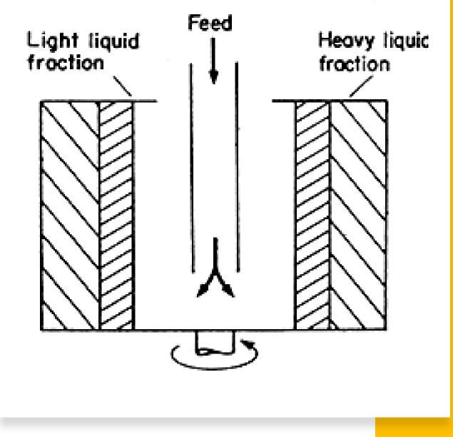
A boundary region between the liquids at a given centrifuge speed forms at a radius  $r_n$  where the hydrostatic pressure of the two layers is equal. This is termed the neutral zone and is important in equipment design to determine the position of feed and discharge pipes. It is found using:
