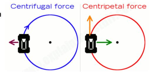
The **centrifugal force** on a particle that is constrained to rotate in a circular path is given by  $F_{\rm c} = mr {\rm w}^2$
