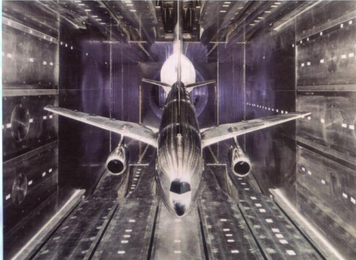
Model aircraft being tested for resonance in a wind tunnel
