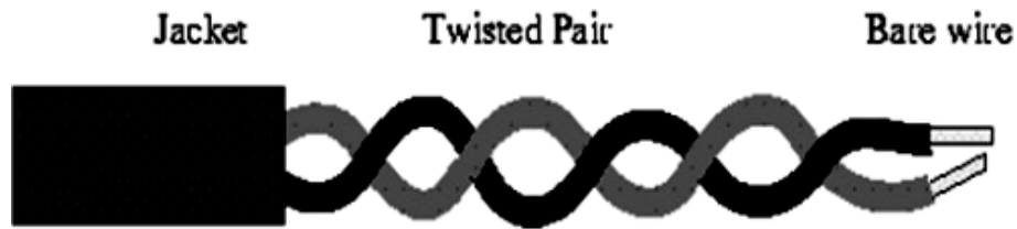
Fig. Unshielded Twisted Pair Cable
