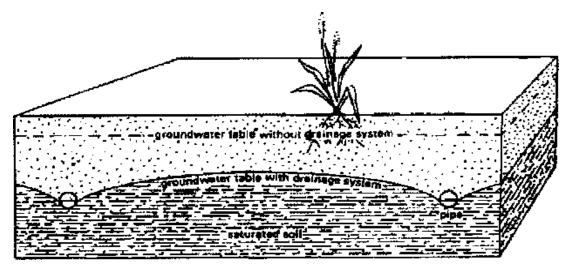
In clay and concrete pipes (30 m long and 5-10 cm in dia.) drainage water enters the pipes through the joints
