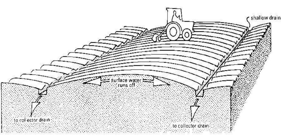
Land forming is mechanically changing the land surface to drain surface water, done by smoothing, grading, bedding or leveling.
