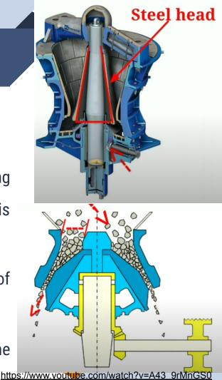
The eccentricity causes the conical crushing head to oscillate between open side setting and closed side setting (OSS and CSS) discharge openings.
