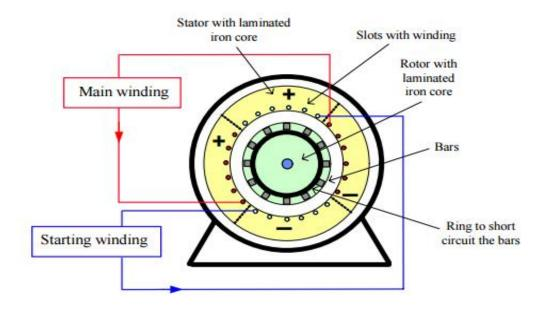
Construction of a single phase induction motor is having squirrel cage rotor, except that the stator is wound for single phase supply. Stator is also provided with a 'starting winding' which is used only for starting purpose.
