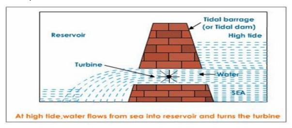
**During low tide,** the sea-water stored in the barrage reservoir is allowed to flow out into the sea. This flowing water also turns the turbines and generates electricity. Thus, as the sea-water flows in and out of the tidal barrage during high and low tides, the turbines rotate continuously to generate electricity.
