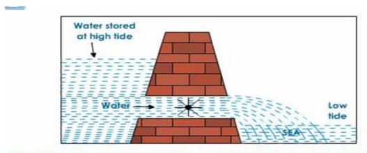
At low tide, stored water flows out from reservoir into sea and turns the turbine
