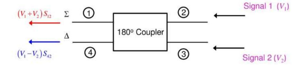
• The signal from the sum port  $\Sigma$  (port 1) is the sum of the input signals 1 and 2.
