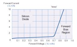
The application of a forward biasing voltage on the junction diode results in the depletion layer becoming very thin and narrow which represents a low impedance path through the junction thereby allowing high currents to flow. The point at which this sudden increase in current takes place is represented on the static I-V characteristics curve above as the "knee" point.
