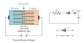
This condition represents the low resistance path through the PN junction allowing very large currents to flow through the diode with only a small increase in bias voltage. The actual potential difference across the junction or diode is kept constant by the action of the depletion layer at approximately 0.3v for germanium and approximately 0.7v for silicon junction diodes.
