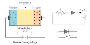
This condition represents a high resistance value to the PN junction and practically zero current flows through the junction diode with an increase in bias voltage. However, a very small reverse leakage current does flow through the junction which can normally be measured in micro-amperes, (  $\mu A$  ).
