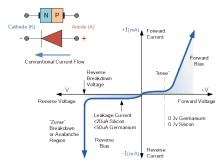
But before we can use the PN junction as a practical device or as a rectifying device we need to firstly bias the junction, that is connect a voltage potential across it. On the voltage axis above, "Reverse Bias" refers to an external voltage potential which increases the potential barrier. An external voltage which decreases the potential barrier is said to act in the "Forward Bias" direction.
