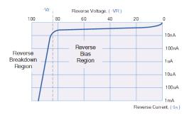
Sometimes this avalanche effect has practical applications in voltage stabilising circuits where a series limiting resistor is used with the diode to limit this reverse breakdown current to a preset maximum value thereby producing a fixed voltage output across the diode. These types of diodes are commonly known as Zener Diodes and are discussed in a later tutorial.
