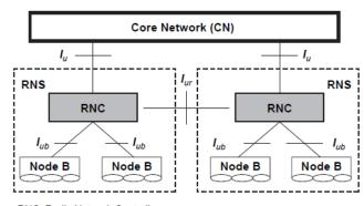
RNC: Radio Network Controller RNS: Radio Network Subsystem
