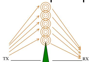
$h_m$  is the height of the obstacle, and  $d_t$  is distance transmitter - obstacle
