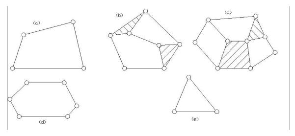
In case, the motion of a link results in indefinite motions of other links, it is a non-kinematic chain. However, some authors prefer to call all chains having relative motions of the links as kinematic chains.
