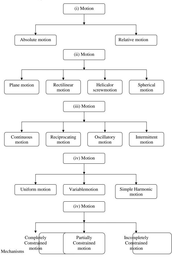
The tree main types of constrained motion in kinematic pair are,
