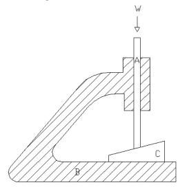
This figure shows the mechanism of a fly press. The element B forms a sliding with A and turning pair with screw rod C which in turn forms a screw pair with A. When link A is fixed, the required fly press mechanism is obtained.
