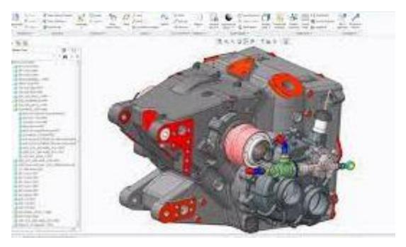
A cursor badge displays when you move the cursor over an object that has constraints applied to it. In the design phase of a project, constraints provide a way to enforce requirements when experimenting with different designs or when making changes. Changes made to objects can adjust other objects automatically, and restrict changes to distance and angle values.
