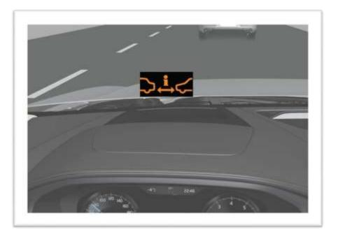
In cars equipped with head-up display, a symbol is shown on the windscreen for as long as the time interval to the vehicle ahead is shorter than the preset value. However, this assumes that the **Show Driver Support** function is activated via the settings in the car's menu system. Distance warning is active at speeds above 30 km/h (20 mph) and only reacts to the vehicle ahead travelling in the same direction. No distance information is provided for oncoming, slow or stationary vehicles.
