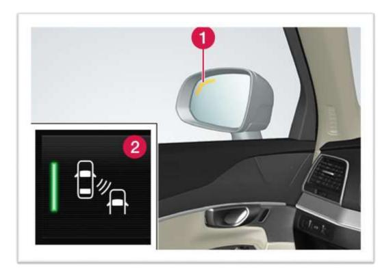
The BLIS function is active at speeds above 10 km/h (6 mph).<u>The system is designed to</u> react when:
