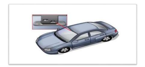
In addition to the camera, lane keeping assist has a steering input assist. Lane keeping assist will gently turn the steering wheel to keep your vehicle between the left and right lane lines, gently steering your vehicle in the opposite direction of the lane boundary. In some systems, the tugging on your steering wheel will become stronger the closer your vehicle gets to the lane markers.
