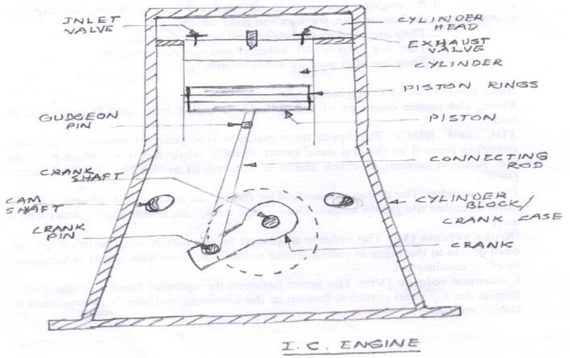
**Compression ratio (rc):** The ratio of the whole cylinder volume (i.e. volume of cylinder when the piston is at BDC) to the clearance volume is called compression ratio. The compression ratio varies from 7:1 to 15:1 for petrol engines and from 16:1 to 22:1 for diesel engines.
