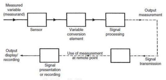
Fig 1.1 Generalised Measurement system
