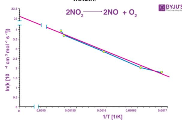
The Arrhenius plot for the decomposition of nitrogen dioxide is illustrated above.
