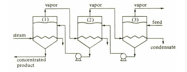
Simplified diagram of backward-feed triple-effect evaporator.
