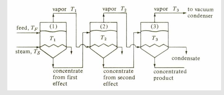
Simplified diagram of forward -feed triple-effect evaporator.
