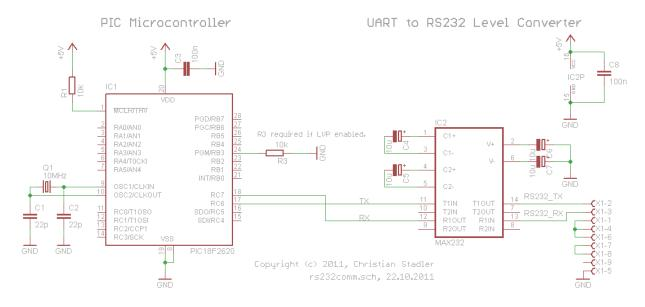
The PIC is running at 10MHz. This will be important later when we configure the baudrate for the serial communication.
