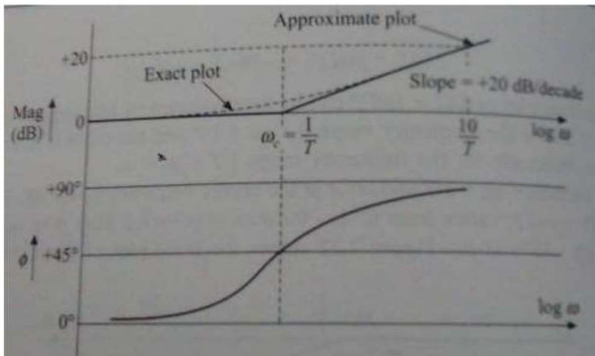
Figure 7.23 Bode plot of the factor  $(1 + j\omega T)$  (simple zero).
