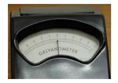
Indicating instrument indicate the instantaneous value of quantity under measurement.
