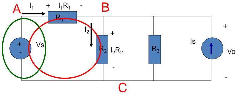
Subtract the voltage rise from C to A through Vs:  $+I_1R_1 + I_2R_2 - Vs = 0$ Notice that the sign of each term matches the polarity encountered 1st
