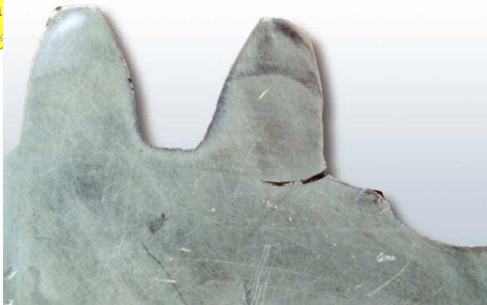
Figure 3. Fatigue Crack in Gear Tooth Root Fillet.
