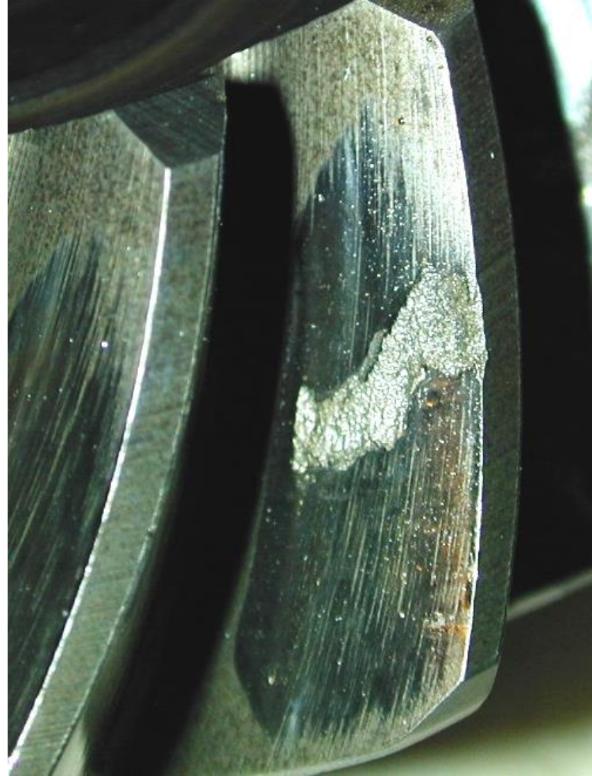
Figure 3. Fatigue Crack in Gear Tooth Root Fillet.
