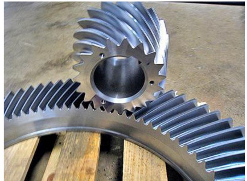
Finished hypoid 38" gear set for a paper pulper cut by 3/16 ball end mill.
