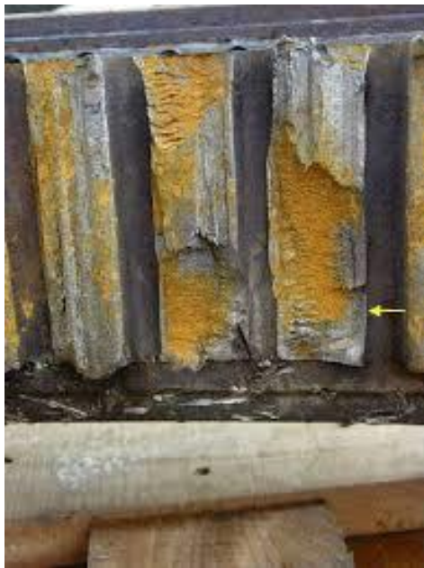
Figure 3. Fatigue Crack in Gear Tooth Root Fillet.
