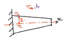
$V_{ans} \sim k_{fw} (T_c - T_s) \over 8$  $\sim h(T_s - T_{so})$
