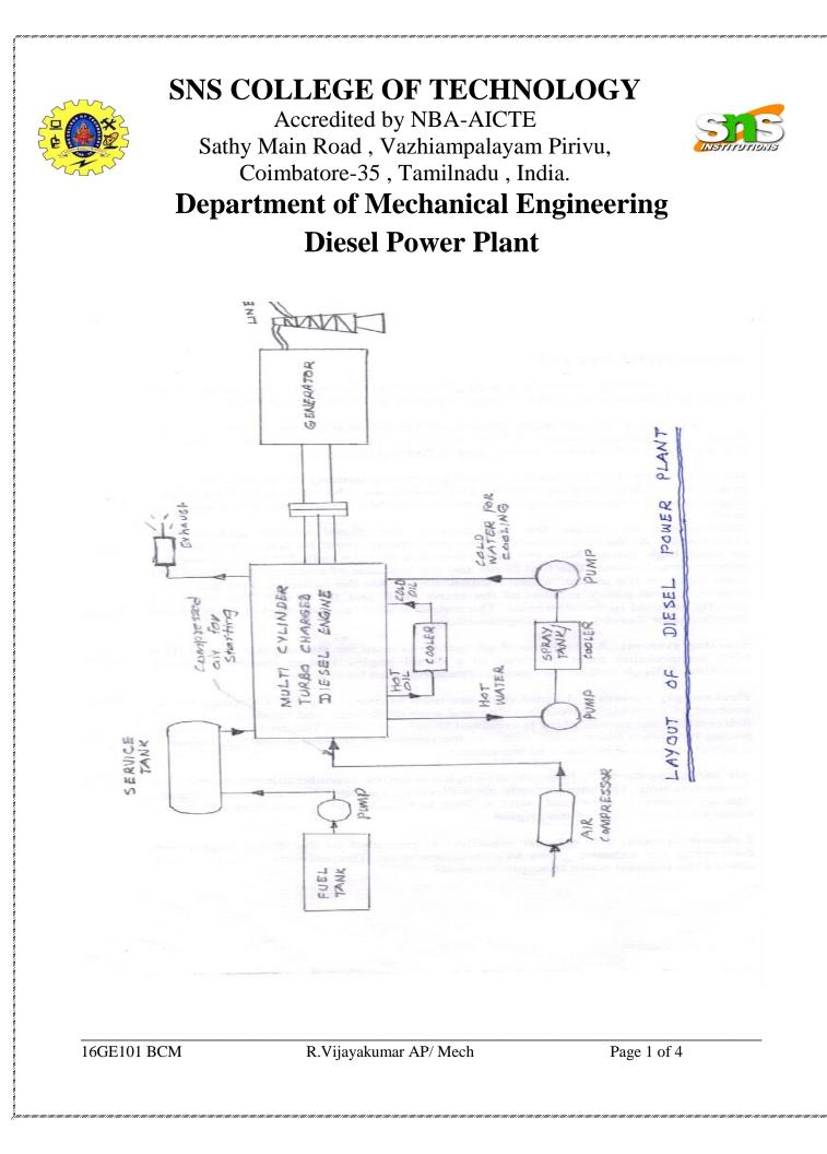
A generating station in which diesel engine is used as the prime mover for the generation of electrical energy is known as Diesel Power Plant.
