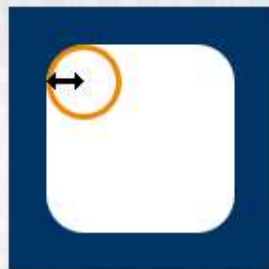
Corners are cut around the corresponding quarters of a circle (or ellipse) with the specified radius.
