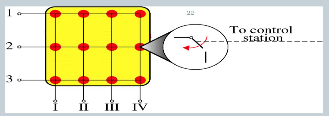
A cross bar switch connects n input lines to m output lines in a grid using micro switches (transistor) at each cross point.
