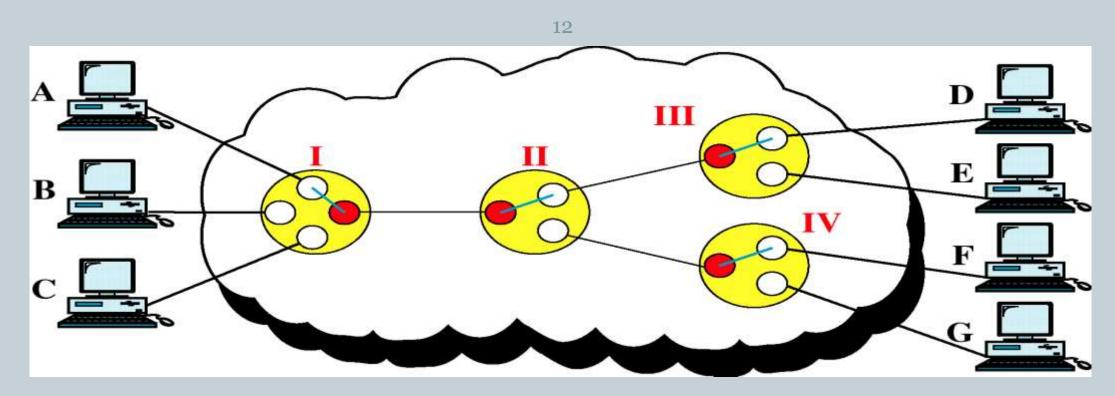
In place of using 3x4=12 point to point connections only 3 switches are used in above figure.
