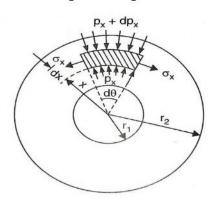
Now consider an elemental spherical shell of radius x and thickness dx as shown in Fig. 18.7. Let  $p_x$  and  $p_x + dp_x$  be the radial pressure at radii x and x + dx respectively. And  $\sigma_x$  is the circumferential tensile stress which is equal in all direction in a spherical shell.
