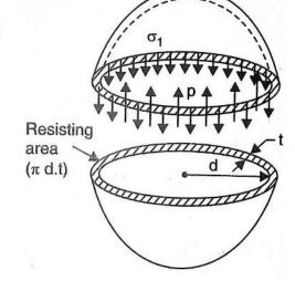
The stress  $\sigma_1$  is tensile in nature The fluid inside the shell is also having tendency to split the shell into two hemispheres along y-y axis. Then it can be shown that the tensile hoop stress will also be equal to  $\frac{pd}{4t}$ . Let the stress is  $\sigma_2$
