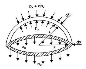
Consider the equilibrium of half of the elementary spherical shell on which the following external force are acting:
