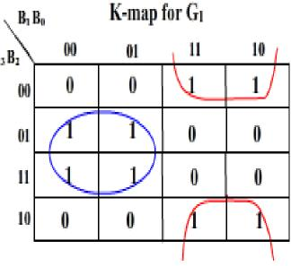
$G_1 = B_1' B_2 + B_1 B_2'$  $G_2 = B_1 \oplus B_2$
