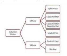
The types of induction motors can be classified depending on whether they are a single phase or three phase induction motor.
