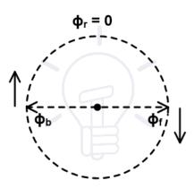
When a motor starts, two fields are induced as shown in the above figure. These two fields are the same magnitude and opposite direction. So, resultant flux is zero. In this condition, the stator field cannot cut by rotor field and resultant torque is zero. So, the rotor cannot rotate but it produces humming.
