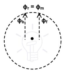
Now consider after the rotation of 90°, both filed are rotated and pointing in the same direction. Therefore, the resultant flux is a summation of both fields.
