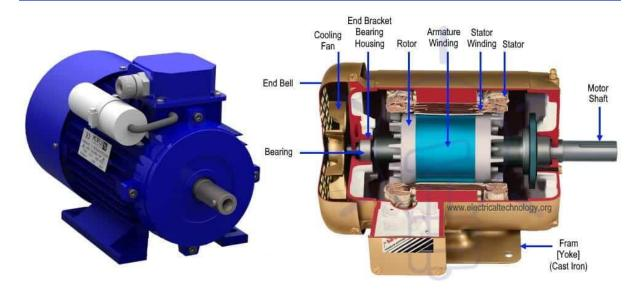
Similar to a three-phase induction motor, single-phase induction motor also has two main parts;
