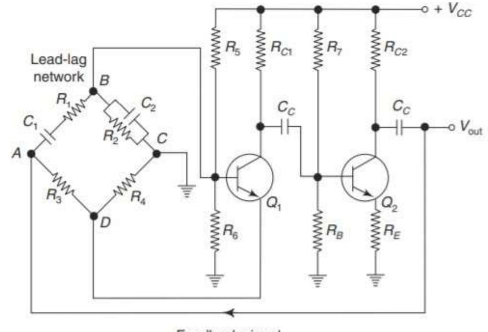
The lead-lag network provides a positive feedback to the input of the first stage and the voltage divider provides a negative feedback to the emitter of Q1.
