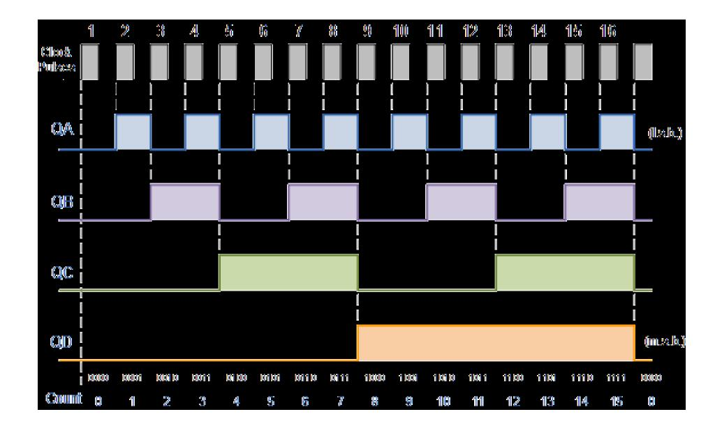
Design of Counters- synchronous up/down counter/ LINEAR AND DIGITAL CIRCUITS/Mr.N.Arunkumar/AP/ECE/SNSCT
