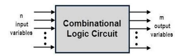
Combinational Logic Circuits are memoryless digital logic circuits whose output at any instant in time depends only on the combination of its inputs.
