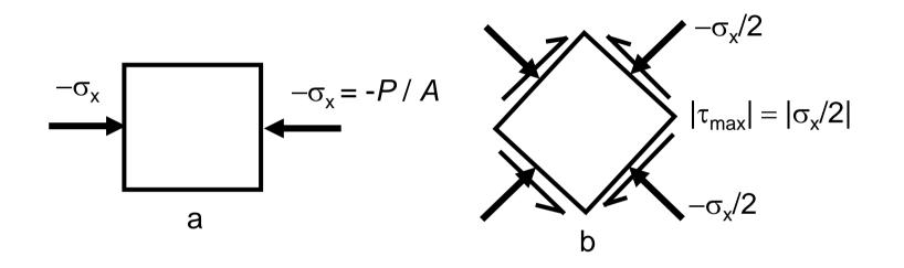
Even though the maximum shear stress in an axially loaded bar is only half the maximum normal stress, the shear stress may cause failure if the material is much weaker in shear than in tension.
