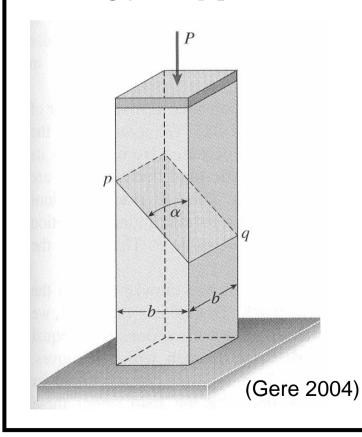
The material is a structural plastic with  $\sigma_{allow}$  (compression) = 7.6 MPa  $\tau_{allow}$  = 4.1 MPa
