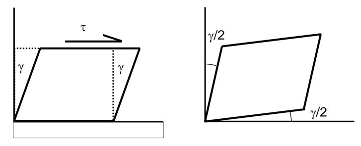
This change in shape is quantified by the angle  $\gamma$ , the shear strain. The angle is measured in radians, **not** degrees.
