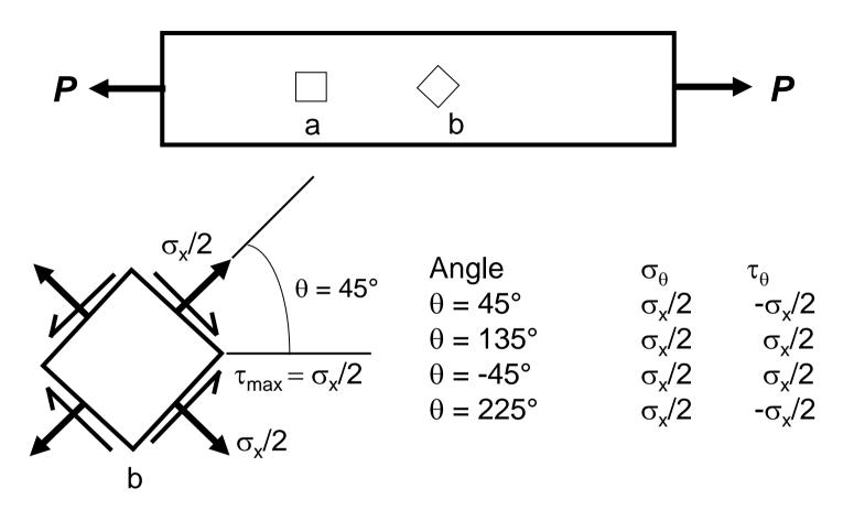
In case b ( $\theta$  = 45°), the normal stresses on all four faces are the same, and all four shear stresses have **equal** and **maximum** magnitude.
