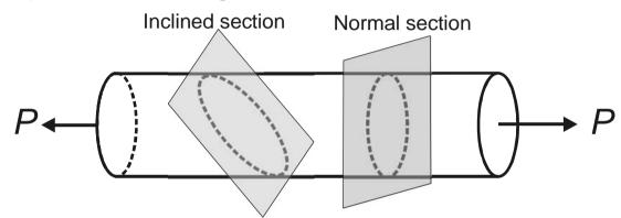
Because the stresses are the same throughout the entire bar, the stresses on the sections are uniformly distributed.
