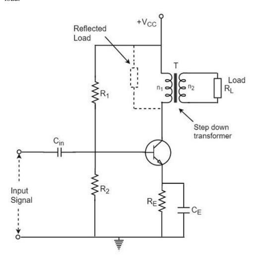
Here  $R_1$  and  $R_2$  provide potential divider arrangement. The resistor Re provides stabilization,  $C_e$  is the bypass capacitor and  $R_e$  to prevent a.c. voltage. The transformer used here is a step-down transformer.
